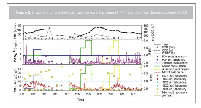
integrated operation of both filtration and biological processes in a MBR plant in order to guarantee nutrient removal.
