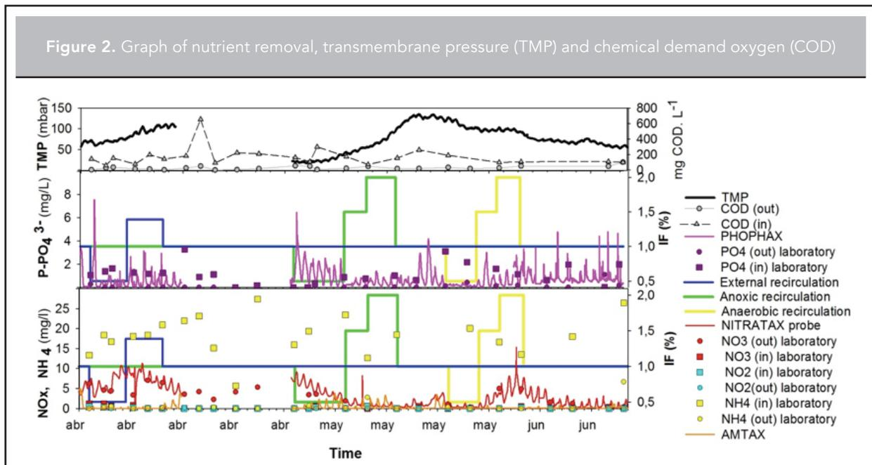
integrated operation of both filtration and biological processes in a MBR plant in order to guarantee nutrient removal.
