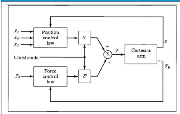
The accommodation strategy concept aims to use force torque data from the assembly action to control the fine motions (Figure 4). Detailed analysis of the force interactions between the parts is necessary so that the error conditions can be recognized directly.
