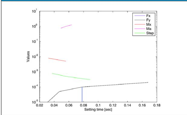
With these values, the control is relatively stable and the response with a tolerance of  $1\text{ mm}$  is  $0.53\text{ s}$ . If we decrease the tolerance, the setting time increases until it becomes unstable in  $1\text{ }\mu\text{m}$  (Figure 11).
