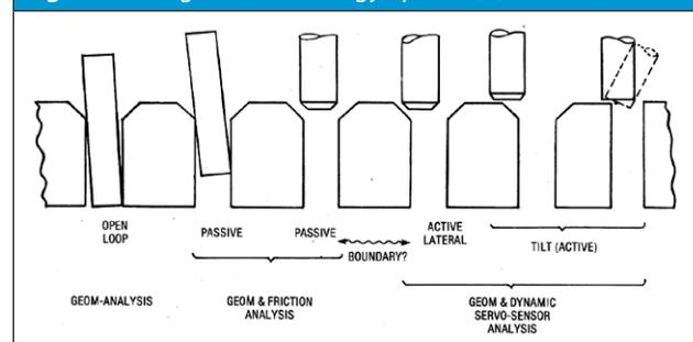
The two kinds of active strategies have been recognized. One is called "logic branching" and the other one "accommodation". Logic branching consists of enumerating the cases of relative position that could occur during the process and
