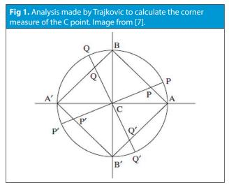
Trajkovic Algorithm has 3 steps. First step is an analysis in low resolution with the aim to extract the most representative points of the image with this condition. In low resolution, it uses the following metric to accept or reject a point as a possible corner:
