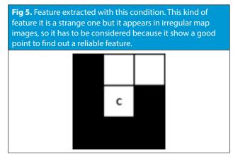
With these simple rules, the algorithm designed for feature extraction by detecting corners, makes a fast search by reducing the workspace since it discards pixels with irrelevant information or pixels with a low value on grayscale. However, discarded pixels are analyzed in other iterations if they are near to a real corner, so it is important because discarded pixel can provide us information that helps to define the appearance of a corner in the image.
