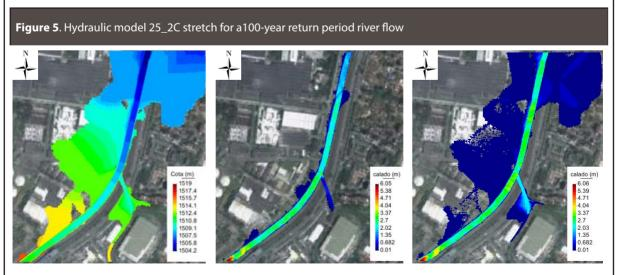
**Figure 5** shows the hydraulic model of a hydrologic flood for a 100-year return period in the 25\_2C stretch. The first image presents the digital elevation map used in the model. The center image presents the water stain in the main channel when it begins to overflow the channel in the flood plain. The image on the right shows the flood stain for the permanent flow of the riverbed for a 100-year return period.
