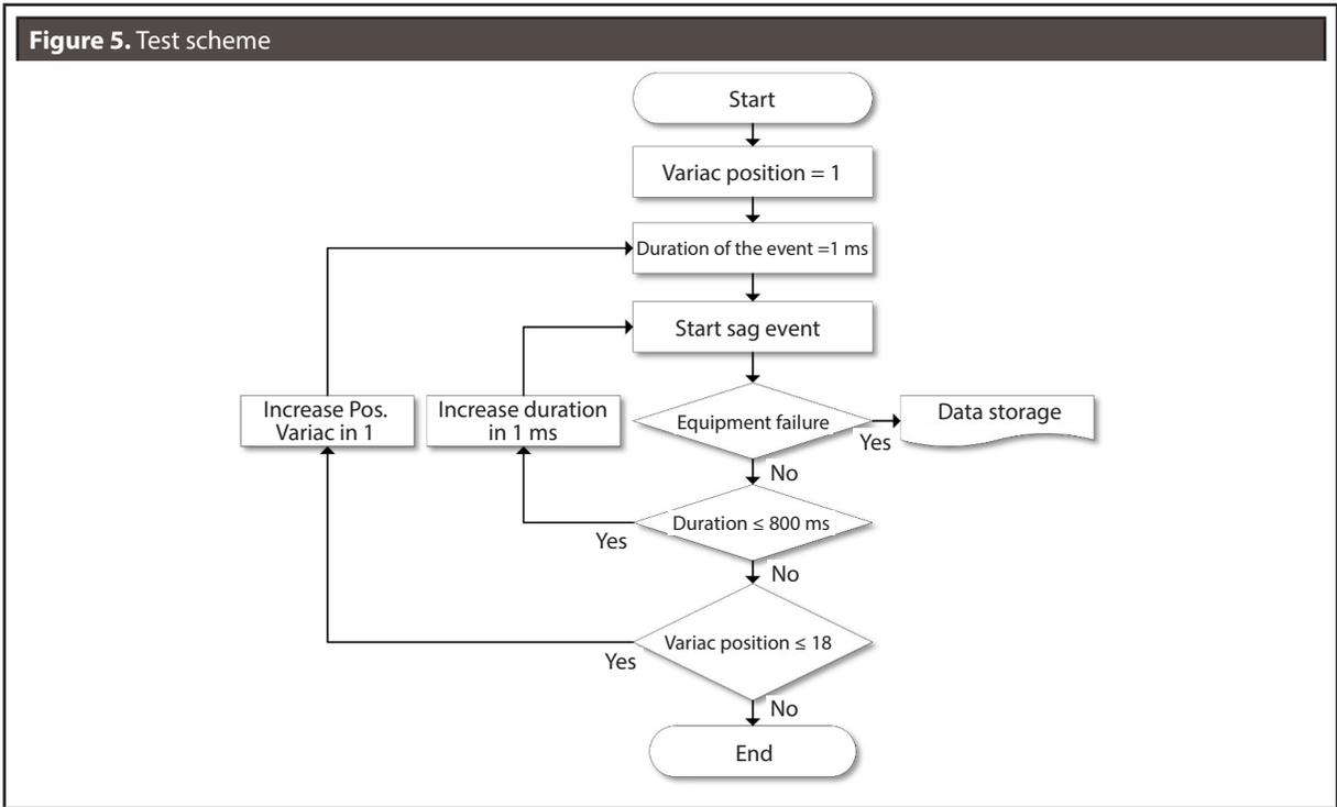
After each power outage of the lamp, there is a wait time of no less than 10 minutes in order to begin the new test. This, for the purpose of stabilizing the functioning of the lamp and allowing for the reestablishment of the ionization and lighting intensity.
