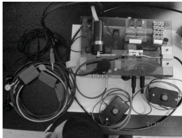
Fig. 8. Final prototype. It shows the electronic components: motor, tension sensor, buttons, EMG circuits (pigs), microphone.
